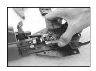
SLIDE LINKAGE MECHANISM AND ADJUSTING ROD (018) SIMULTANEOUSLY FROM COLLAR (006)
