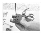
LOOSEN SCREWS (532) WITH 3 MM HEXAGON WRENCH KEY. CHANGE TEETH ONE AT A TIME TO PREVENT REVERS TEETH.
