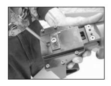
TURN ADJUSTING ROD (018)180°WITH A SCREW DRIVER TO THE DESIRED ADJUSTMENT.
