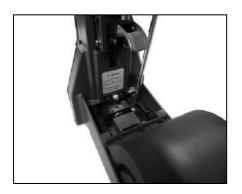
IF WANT TO SHOOT LONG LEG STAPLES. LOOSEN ROUND HEAD SCREW (542) WITH SCREW DRIVER. MOVE RIGHT COIL GUIDE (017) AND LEFT COIL GUIDE (038) OUT. THEN SET ROUND SCREW (542).
