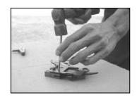
LOOSEN SCREWS (535) WITH 3 MM HEXAGON WRENCH KEY. TAKE OFF THE SPRING PIN (537) WITH HAMMER AND 6 MM STRAIGHT ROD.
