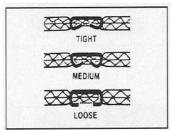
USE ROD(DIA 3 MM) OR 2.5G MM HEXAGON WRENCH KEY. TURN COLLAR (006) THROUGH WINDOW CLOCKWISE TO TIGHTEN CLINCH AND COUNTER-CLOCKVIDE TO LOOSEN CHINCH.
