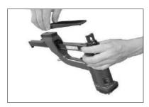
Assemble the new *Anvil (029)* and *Screws (512,514)*.
