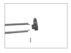
Separate *Springs(022)* and *Block(028)* by taking away *Rod(025)*.
