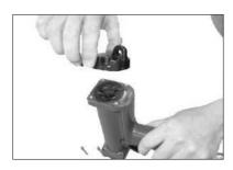
Release *Screws(501)* and take away *Cap(001)*, *Packing(002)* and *Bumper(003)*.
