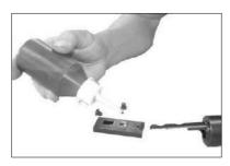
Reassemble New Driver Guide (016) and *Screws*(520).
