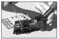
LOOSEN SCREWS (510) WITH 3 MM HEXAGON WRENCH KEY.
