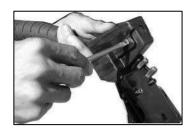
LOOSEN PIVOT SCREW (006) WITH FLAT SCREW DRIVER. REMOVE HANDLE (002) AND LINKAGE MECHANISM.
