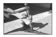
REMOVE SPRING PIN (501) WITH HAMMER AND 5 MM STRAIGHT ROD.
