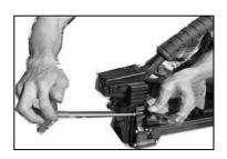
LOOSEN SCREWS (508, 509) AND NUT (520) WITH 8 MM SPANNER AND 4 MM HEXAGON WRENCH KEY.
