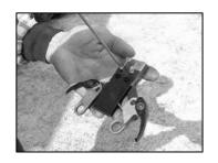
LOOSEN SCREWS (513) WITH 3 MM HEXAGON WRENCH KEY. TAKE OFF THE SPRING PIN (515) WITH HAMMER AND 6 MM STRAIGHT ROD.
