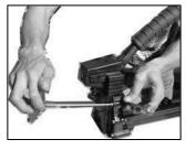
LOOSEN SCREWS (508,509) AND NUT (520) WITH 8 MM SPANNER AND 4 MM HEXAGON WRENCH KEY.
