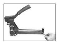
PULL PUSHER (036) BACK UNTIL IT STOPS ON PUSHER PIVOTS(032)THEN ROTATE PUSHER(036)TO POSITION.
