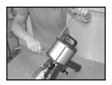
REMOVE SCREWS (501) AND NUT (515) WITH 10 mm SPANNER AND 5 mm HEXAGON WRENCH KEY.
