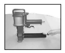
PULL PUSHER (046) BACK UNTIL IT STOPS ON PUSHER GUIDE (043,045) THEN ROTATE PUSHER (046) TO POSITION.
