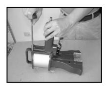
REMOVE TWO SCREWS (513) CONNECT WITH CAP (001) WITH 6mm HEXAGON WRENCH KEY.
