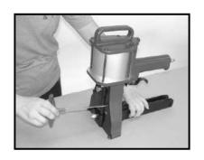
LOOSEN SCREWS (506) WITH 5  ${\tt mm}$  HEXAGON WRENCH KEY .
