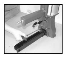
LOOSEN AND REMOVE SCREWS (523) WITH 4mm HEXAGON WRENCH KEY.
