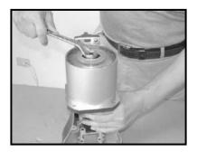
REMOVE LOCK NUT (502) WITH 17mm SPANNER THEN YOU CAN TAKE OUT PISTON.
