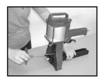
LOOSEN SCREWS ( 506 ) WITH  $5\,\mathrm{mm}$  HEXAGON WRENCH KEY .
