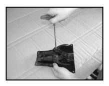
LOOSEN SCREWS (526) WITH 4 mm HEXAGON WRENCH KEY.
