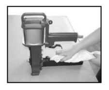
REMOVE TAR BUILDUP WITH KEROSENE #2 FUEL OIL OR DIESEL FUEL . DO NOT ALLOW SOLVENT TO GET INTO THE CYLINDER OR DAMAGE MAY OCCUR . DRY OFF THE TOOL COMPLETELY BEFORE USE
