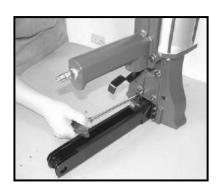
LOOSEN SCREWS (523) WITH 4  ${\tt mm}$  HEXAGON WRENCH KEY .
