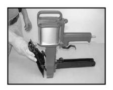
REMOVE THE FRONT PLATE (019) ASSEMBLY AND CLINCHER(034) ASSEMBLY.
