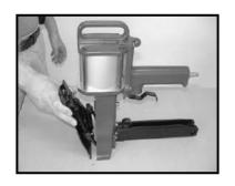
REMOVE THE FRONT PLATE (019) ASSEMBLY AND CLINCHER (034) ASSEMBLY.
