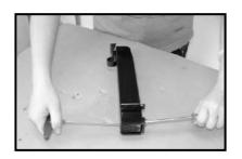
LOOSEN SCREW (518) AND NUT (519) WITH 2.5 mm HEXAGON WRENCH KEY AND 7 mm SOCKET WRINCH .
