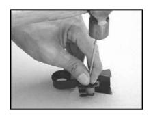
REMOVE SPRING PIN (525) WITH HAMMER AND 4 mm (DIA) STRAIGHT ROD.
