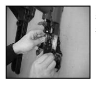
SLIDE LINKAGE MECHANISM AND ADJUSTING ROD (018) SIMULTANEOUSLY FROM COLLAR (006).
