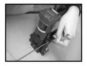
LOOSEN SCREWS (530 , 531) AND NUT (542) WITH 8 mm SPANNER AND 4 mm HEXAGON WRENCH KEY .
