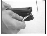
LOOSEN ROD (032) WITH 6 mm OFFSET WRENCH REMOVE PUSHER GUIDES (033). REMOVE PUSHER (030)
