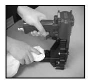
REMOVE TAR BUILDUP WITH KEROSENE #2 FUEL OIL OR DIESEL FUEL . DO NOT ALLOW SOLVENT TO GET INTO THE CYLINDER OR DAMAGE MAY OCCUR . DRY OFF THE TOOL COMPLETELY BEFORE USE .
