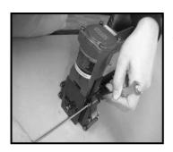
LOOSEN SCREWS( 530,531 ) AND NUT( 542 ) WITH 8  ${\rm mm}\,$  SPANNER AND 4  ${\rm mm}\,$  HEXAGON WRENCH KEY .
