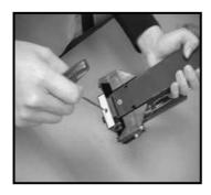
LOOSEN SET SCRCW (526) WITH 3 mm HEXAGON WRENCH KEY.
