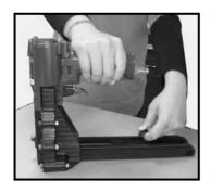
PULL PUSHER (036) BACK UNTIL IT STOPS ON PUSHER PIVOTS (032) THEN ROTATE PUSHER (036) TO POSITION .
