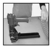
DISCONNECT THE AIR SUPPLY FROM THE TOOL.
