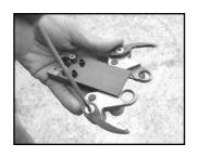
LOOSEN SCREWS (532) WITH 3  ${\tt mm}$  HEXAGON WREM KEY . CHANGE TEETH ONE AT A TIME TO PREVENT REVERS TEETH .
