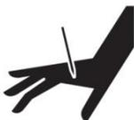
Keep hands and body away from the discharge area of the tool. A contact arm tool may bounce from the recoil of driving a fastener and an unwanted second fastener may be driven, possibly causing injury.
