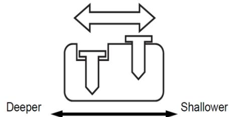
1. With air pressure set, drive nails into a representative material sample to determine if adjustment is necessary.
