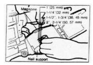
Nail length adjustment: The nail support can be moved
