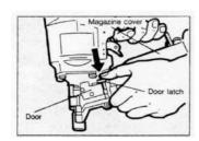
**Open the magazine:** Pull down door latch and swing door
