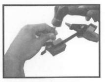
Take away two spring pins (517) withΦ2.3mm rod and hammer.
