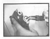
Take away C-Ring(530), front valve seat(019) and valve(020) with pliers.
