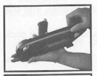
Insert c-rings into your tool following the instructions of loading the tool.
