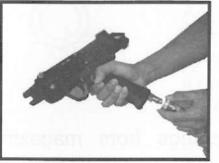
1. Disconnect the air supply from the tool.
