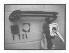
Push piston rod (026) up. Take away nut (524) with M10 Spanner and pliers. Then, take away toothed lock washer-external (527), washer (038), piston (003) and piston rod (026).
