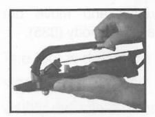
Disconnect the air supply and move out remnant c-rings from magazine body (035).
