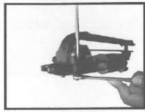
Loosen Screw (516) and nut (515) with M5 Hex. Wrench key and M10 spanner.
