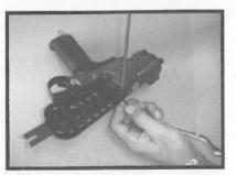
Take away screw (523), nut (514) and side plates (015) with M4 Hex. Wrench key and M8 Spanner.
