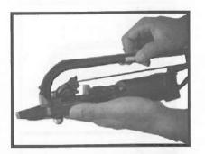
Disconnect the air supply and move out remnant c-rings from magazine (035).
