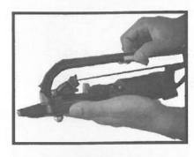
Disconnect the air supply and move out remnant c-rings from magazine body (035).
