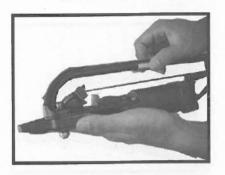
Disconnect the air supply and move out remnant c-rings from magazine body(035).
