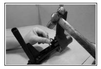
Take away spring pin (519) with  $\,\phi$  5mm shaft and hammer.
