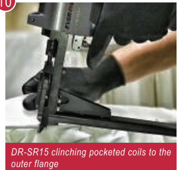
ECAR Stapling foundation spring to flat members
