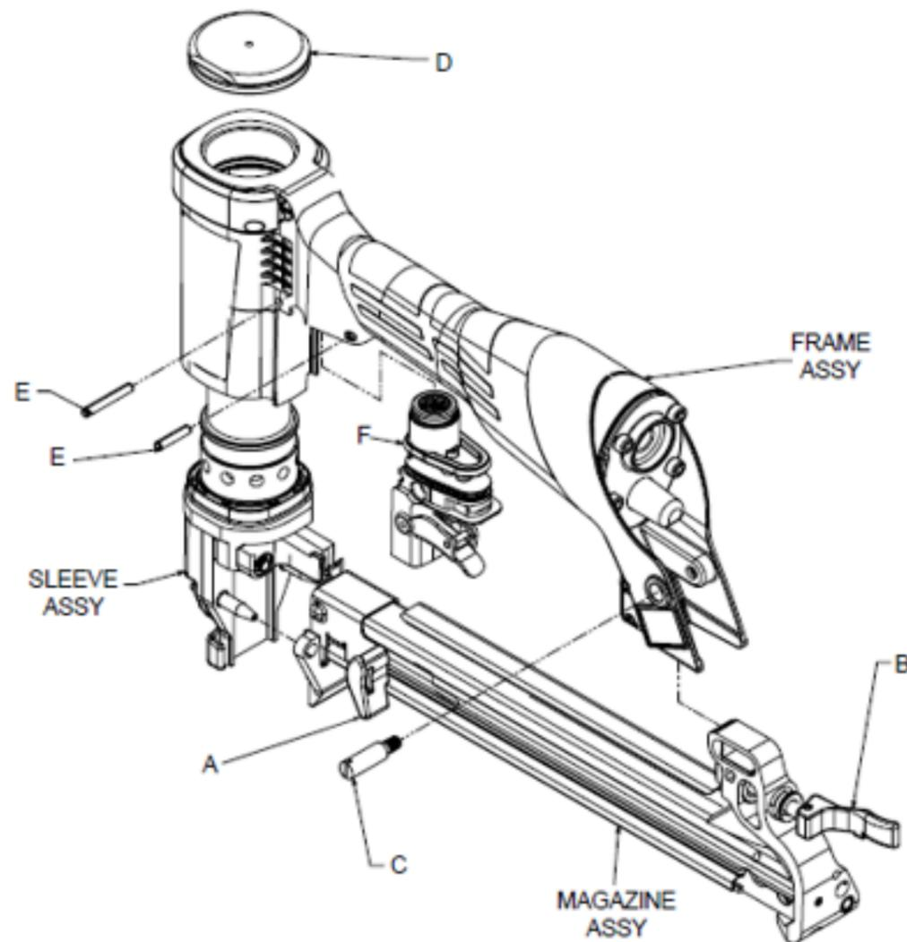
1. Disconnect the air line from the tool. Remove all staples from the magazine and position the pusher(A) to the front of the magazine.
