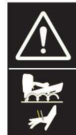
Keep hands and body away from the discharge area of the tool. A contact arm tool may bounce from the recoil of driving a fastener and an unwanted second fastener may be driven, possibly causing injury.
