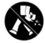
The connector on the tool must not hold pressure when air supply is disconnected. If a wrong fitting is used, the tool can remain charged with air after disconnecting and thus will be able to drive a fastener even after the air line is disconnected, possibly causing injury. Do not pull trigger or depress contact arm while connected to the air supply as the tool may cycle, possibly causing injury.
