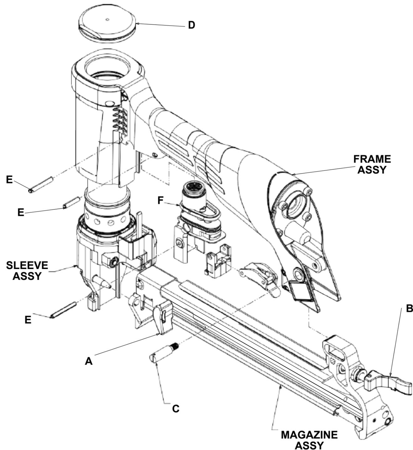
1. Disconnect the air line from the tool. Remove all staples from the magazine and position the pusher(A) to the front of the magazine.
