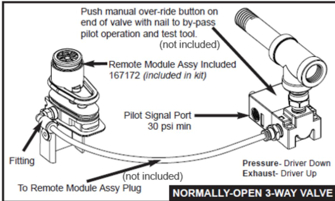
A 3-way normally open pilot operated valve is not included with this ETVA12-RF kit. Other electrical operated valves may be ordered separately as follows:
