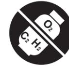
DO NOT USE OXYGEN, COMBUSTIBLE GASES, OR BOTTLED GASES AS A POWER SOURCE FOR THIS TOOL AS TOOL MAY EXPLODE, POSSIBLY CAUSING INJURY.
