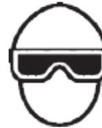
The employer and/or user must ensure that proper eye protection is worn. Eye protection equipment must conform to the requirements of the American National Standards Institute, ANSI Z87.1 and provide both frontal and side protection. NOTE: Non-side shielded spectacles and face shields alone do not provide adequate protection.
