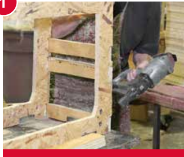
SN50S5 assembling a chair frame
