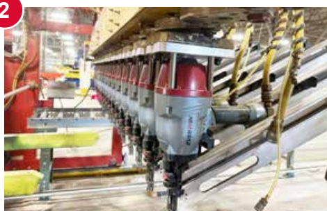
Automation: FSN3490 on a wallpanel bridge
