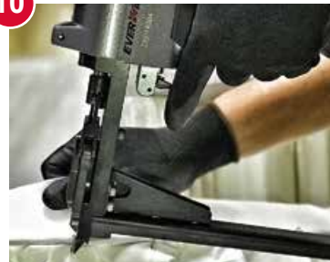
DR-SR15 clinching pocketed coils to the outer flange
