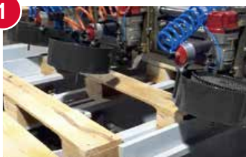
Automation: PN70PAL nailing decks to blocks
