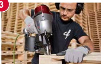
PN90 nailing bottom decks to pallet blocks
