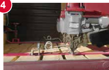
Automation: PN80PAL nailing decks to stringers
