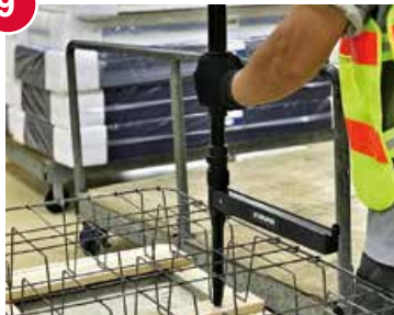
ECAR Stapling foundation spring to flat members
