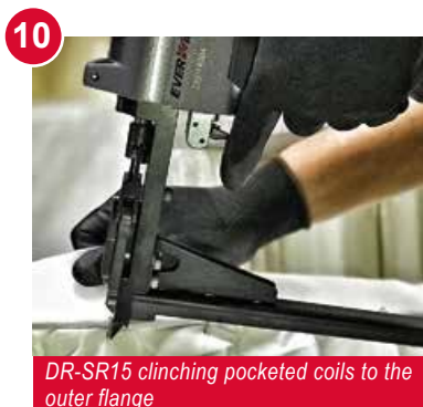
ECAR Stapling foundation spring to flat members
