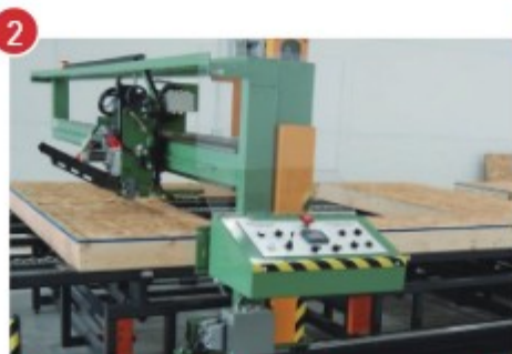
Automation: FSN2283 on a wallpanel bridge
