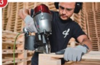
PN90 nailing bottom decks to pallet blocks
