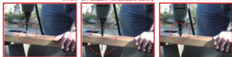
1. Aim 2. Actuate retractable safety 3. Shoot to remove nail
