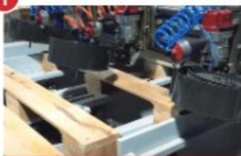
Automation: PN70PAL nailing decks to blocks
