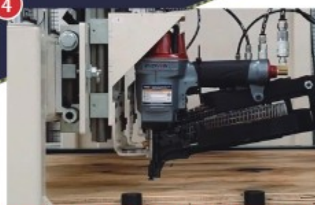
Automation: PN80PAL-JM at a sheathing station
