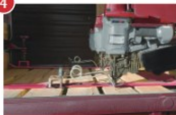
Automation: PN80PAL nailing decks to stringers
