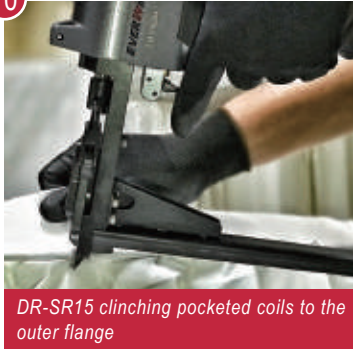
ECAR Stapling foundation spring to flat members
