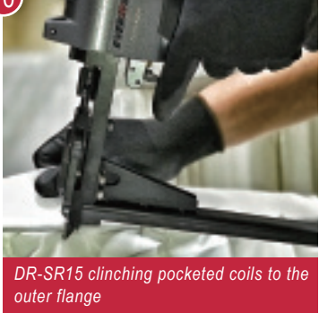
ECAR Stapling foundation spring to flat members
