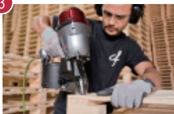
PN90 nailing bottom decks to pallet blocks
