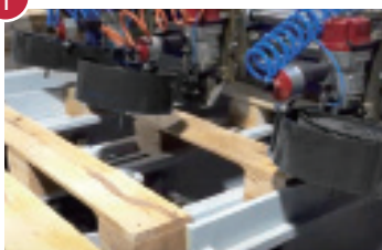
Automation: PN70PAL nailing decks to blocks
