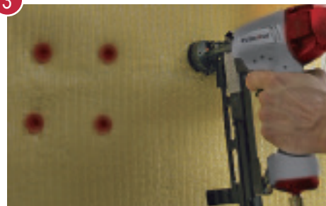
FS9240BC securing insulation layers
